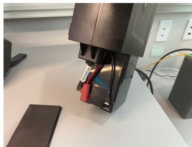
5. Turn the unit upside down over a soft surface and allow the battery to slide out.
